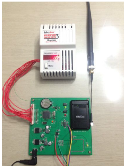
Figure 2. Connection of Siren Pro 3 and WCDMA module
